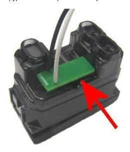
The black connection wire 'PB' of the LED is combined with one of the eight pushbutton connection wires. The white connection wire 'C' of the LED is combined with the common connection wire 'COM' for the pushbuttons.
