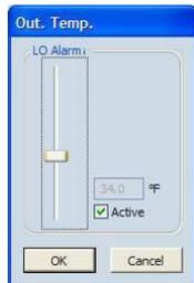
Move the slider control up to increase the alarm trigger value, and down to decrease the trigger value. Click the “Active” checkbox to enable the alarm, click the Ok button, and you’re all set! The alarm icon will appear green to indicate that it is active.
