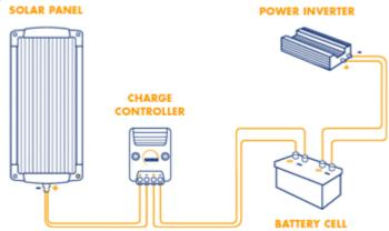
Composed of multiple solar cells in series or in parallel, a solar panel produces direct current (DC) power; when a solar panel is connected to a battery, this power is stored in the battery. A charge controller connected between the solar panel and the battery monitors the battery and prevents the solar panel from overcharging the battery while assuring a complete charge.
