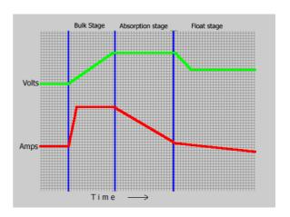
The brighter the sunlight, the more voltage the solar cells produce. This excessive voltage could damage the batteries. A charge controller is used to maintain the proper charging voltage on the batteries. As the input voltage from the Solar panels array rises, the charge controller regulates the charge to the batteries preventing overcharging.
