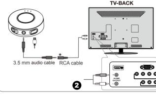
\*Find the correct ANALOG output: You can connect wired earphones with the RCA cable to test whether the sound is normal.
