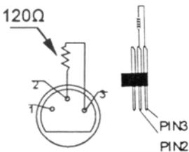
A DMX terminator is recommended for installations where the DMX cable has to run a long distance or is in an electrically noisy environment (e.g. discos). The terminator prevents corruption of the digital control signal by electrical noise. The DMX terminator is simply an XLR plug with a 120Ω resistor between pins 2 and 3, which is then plugged into the XLR output socket of the last device in the chain. Please see illustrations.
