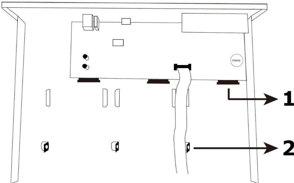
2. Get a compatible hard disk. With the PCB side facing down, insert the hard disk in one of the hard disk connectors.
