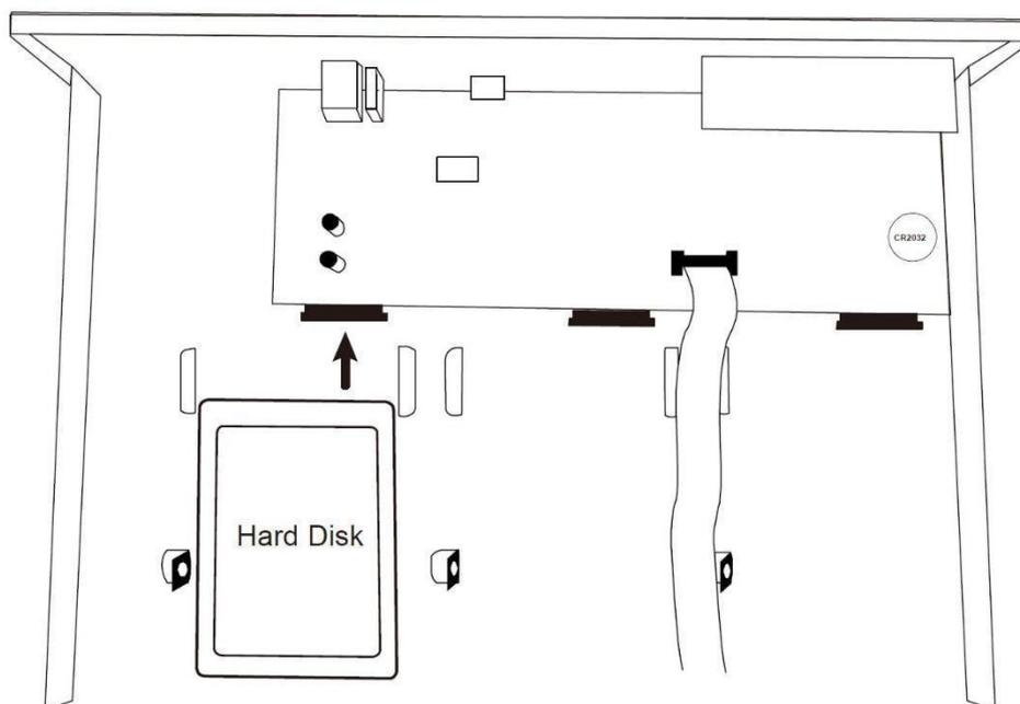
3. Fasten the hard disk to the bracket by securing the screw on the bracket.
