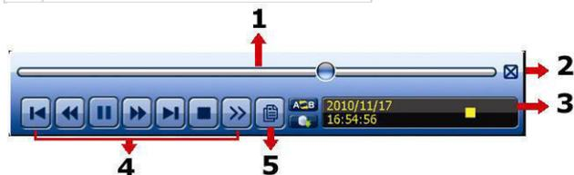
**Note:** There must be at least 8192 images of recorded data for playback to work properly. If not, the device will stop playback. For example, if the IPS is set to 30, the recording time should be at least 273 seconds (8192 images / 30 IPS) for the playback to work properly.
