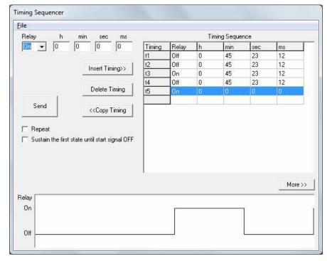
By selecting the option 'auto start & repeat', the timing sequence restarts automatically when the power supply is connected or when there has been a power outage.
