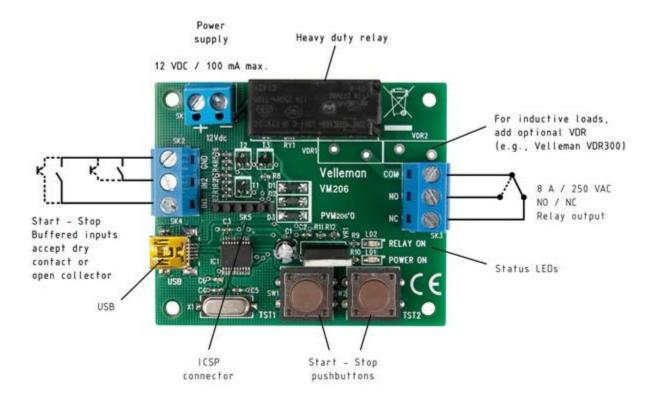
You can disconnect the USB cable and test the timer operation as a stand-alone device with the 12 V supply.
