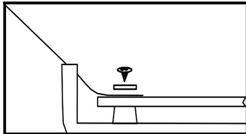
Fix the screen foil using a washer and screw. (Push the screw through the foil)
